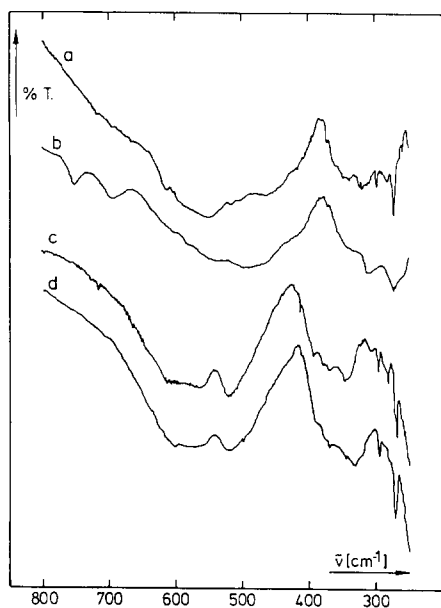
Fig. 4. IR spectra of \text{Sr}_3\text{NpO}_6 (spectrum a), \text{Sr}_3\text{UO}_6 (spectrum b), \text{Ca}_3\text{NpO}_6 (spectrum c) and \text{Ca}_3\text{UO}_6 (spectrum d).
